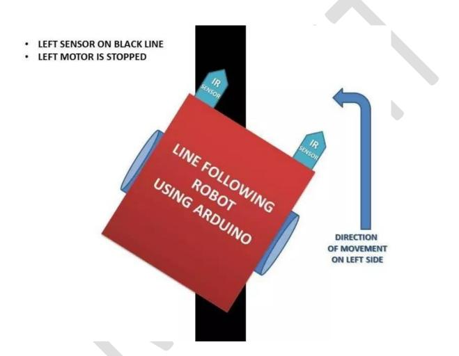
When LEFT IR Sensor Goes on Black Line then It will not receive any signal and the other IR Pair which is on the white surface will receive the signal (same as Previously) and it will make the motor of the left side to be stopped and the motor from the right side will be in the forward direction and that will produce turn on the left side.
