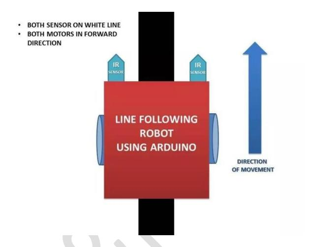
When Line goes straight, we must make IR pairs in such manner that it will be on the white surface and our motors will move in the Forward Direction.
