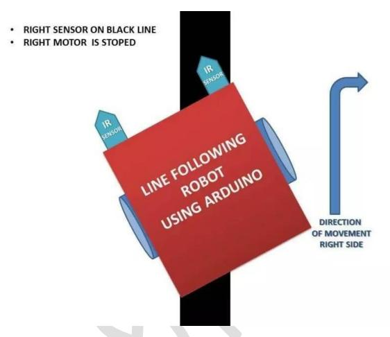
When Right IR Sensor Goes On Black Line then It will not receive any signal and the other IR Pair which is on the white surface will receive the signal and make the motor of right side to be stopped and the motor from the left side will be in the forward direction and that will produce turn on the right side.
