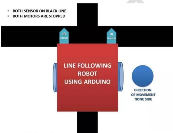
If both sensors are on the black line, then they won't receive any signal so both the motors should stop.
